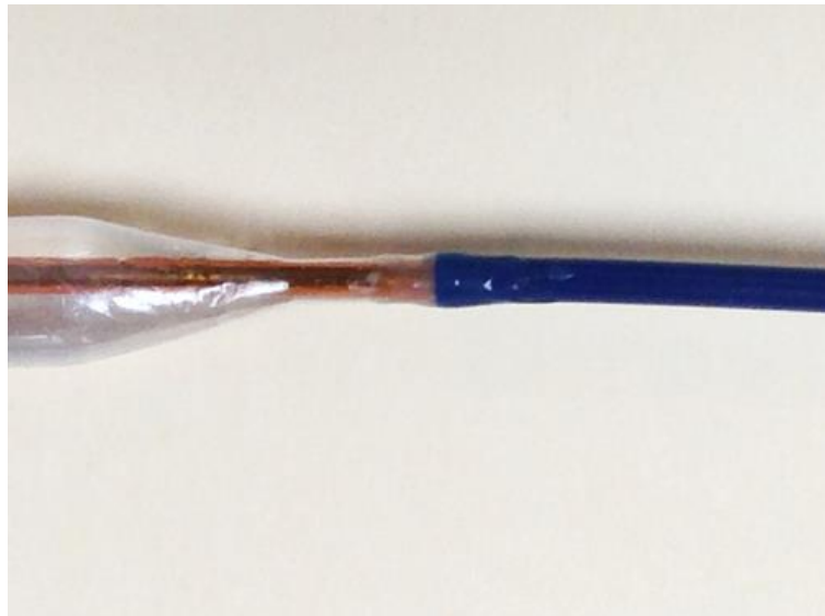
A balloon catheter from Interface Catheter Solutions is assembled using a Cyberbond adhesive. (Photo courtesy of Interface Catheter Solutions.)
